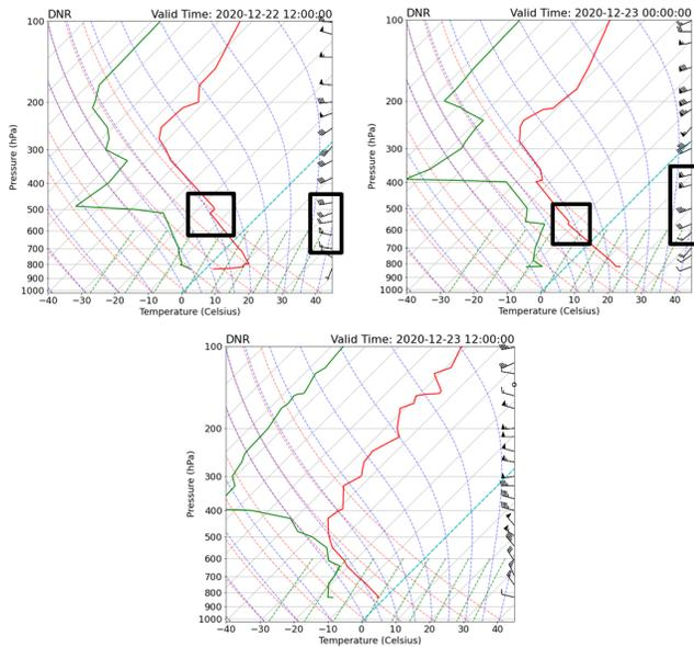
**Figure 10.** Denver, Colorado soundings from 12 UTC 22 December 2020 to 12 UTC 23 December 2020 at 12 h intervals. The black boxes isolate the inversion layer and the wind shear above 600 hPa supportive of the development of a bora. The lack of these ingredients in the third sounding aligns with the end of the bora across the Colorado Front Range.
