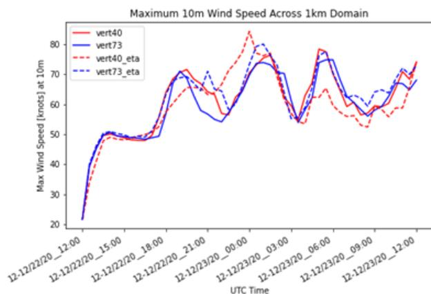
**Figure 16.** The maximum 10 m wind speed across the 1 km innermost domain as a function of time for each WRF simulation.
