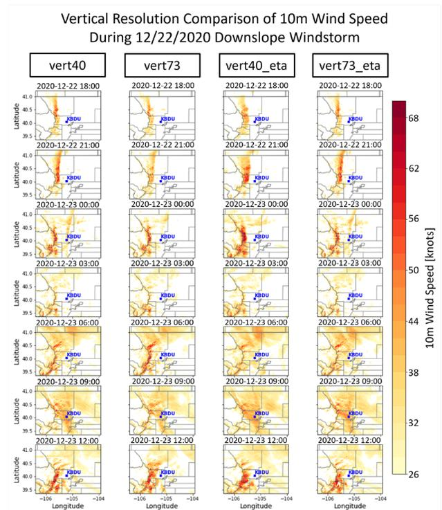
**Figure 14.** Spatial comparison of the 10-m wind speed for the four WRF simulations (from left to right: 40 vertical levels, 73 vertical levels, 40 eta levels, and 73 eta levels). The chinook windstorm is characterized by the localized stronger winds immediately along the Colorado Front Range. After 0000 UTC 23 December 2020, the stronger wind speeds become more widespread following the passage of an upper-level trough, transitioning the chinook into a bora.
