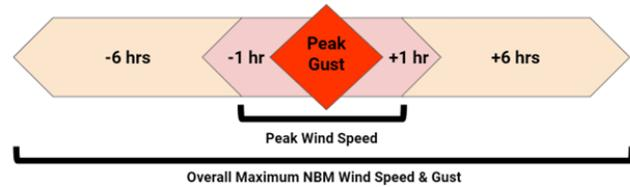
**Figure 2.** Schematic summarizing the methods used to determine the peak wind speed and gust associated with each windstorm within the NBM forecasts.
