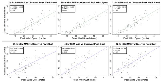
**Figure 4.** Scatter plots of the mean absolute errors (MAEs) of NBM forecasts compared with observed peak wind speeds and gusts. The first row is the MAE of wind speeds, and the second row is the MAE of wind gusts. The columns identify the errors for various forecast lead times (left-to-right: 24 hr, 48 hr, and 72 hr). The linear fit lines for the wind speeds and gusts (green and blue lines, respectively) show a direct relationship between the NBM MAE and the observations.
