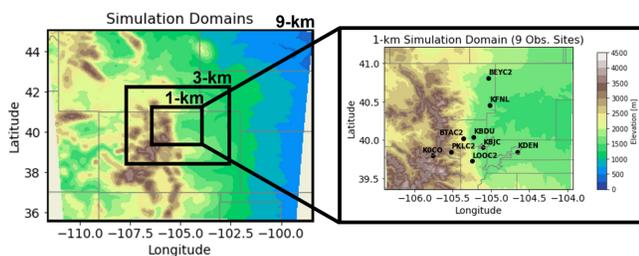
**Figure 3.** WRF domains used to simulate the 22 December 2020 downslope windstorm across the northern Colorado Front Range. The domains consist of one larger, 9 km resolution domain and two nested domains (3 km and 1 km resolutions), shown on the left. The innermost 1 km domain is shown to the right. The black dots represent the 10 observational sites used in this study.
